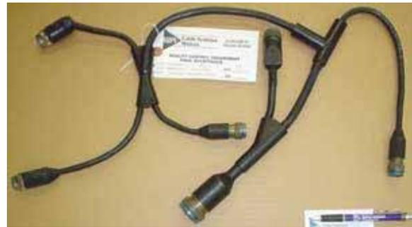
**FIGURE 2.** This combined harness is an example of a harness that can be used to connect multiple units together in a benign environment.
