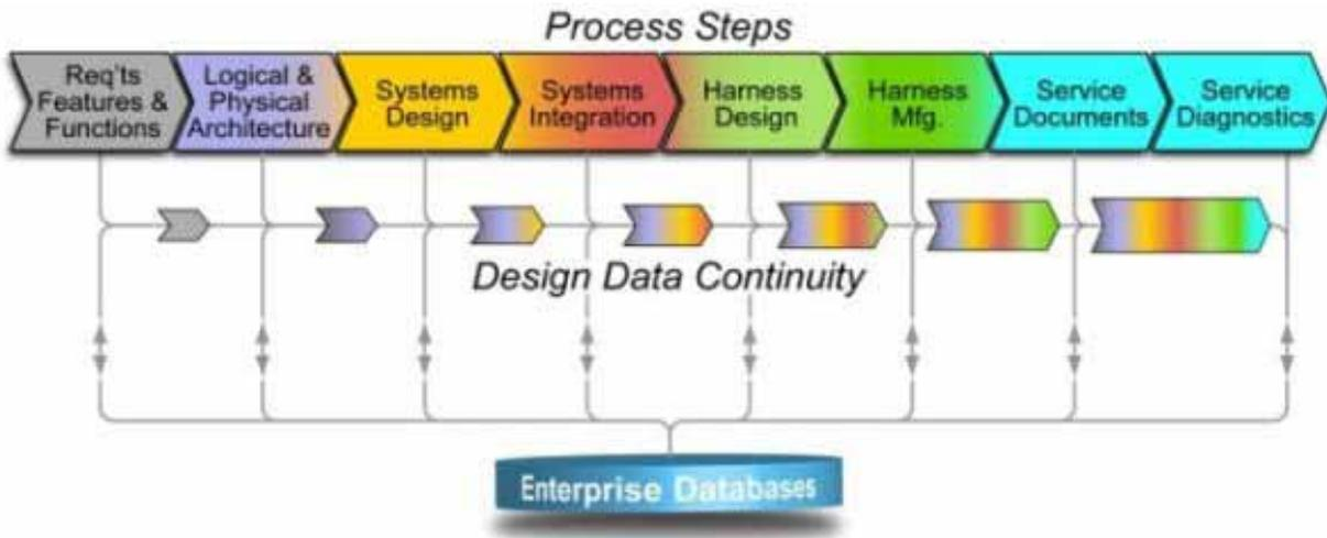
**Figure 1:** Digital continuity implies a series of smooth transitions among all the steps of the design flow. Each process step (stage) contributes data to the subsequent steps. This information is preserved and reused, maturing as it moves ahead in the process.
