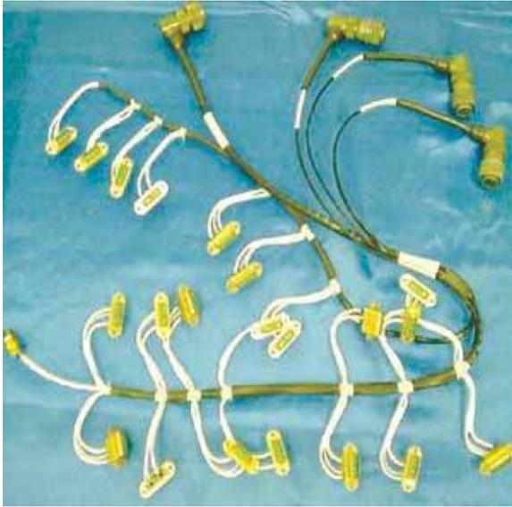
**FIGURE 1.** An open harness is most commonly used for internal wiring of units.
