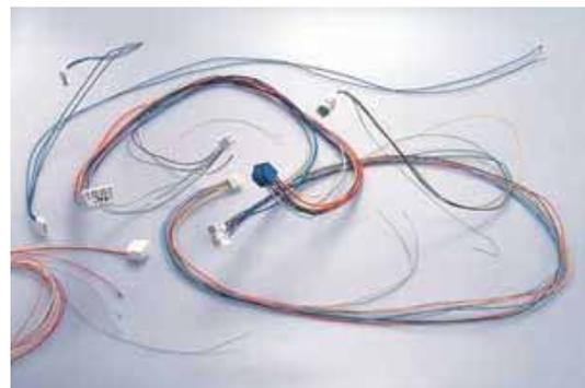
**FIGURE 2.** These wire harnesses were produced on a fully-automatic machine.
