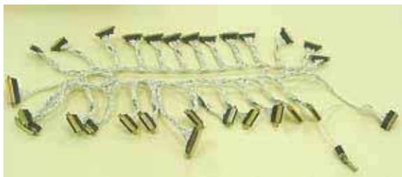
**FIGURE 3.** The molded harness is fully protected and suitable for use in harsh environments where it may be exposed to moisture, dirt and other hazards. It is abrasion resistant and will not degrade when handled roughly.
