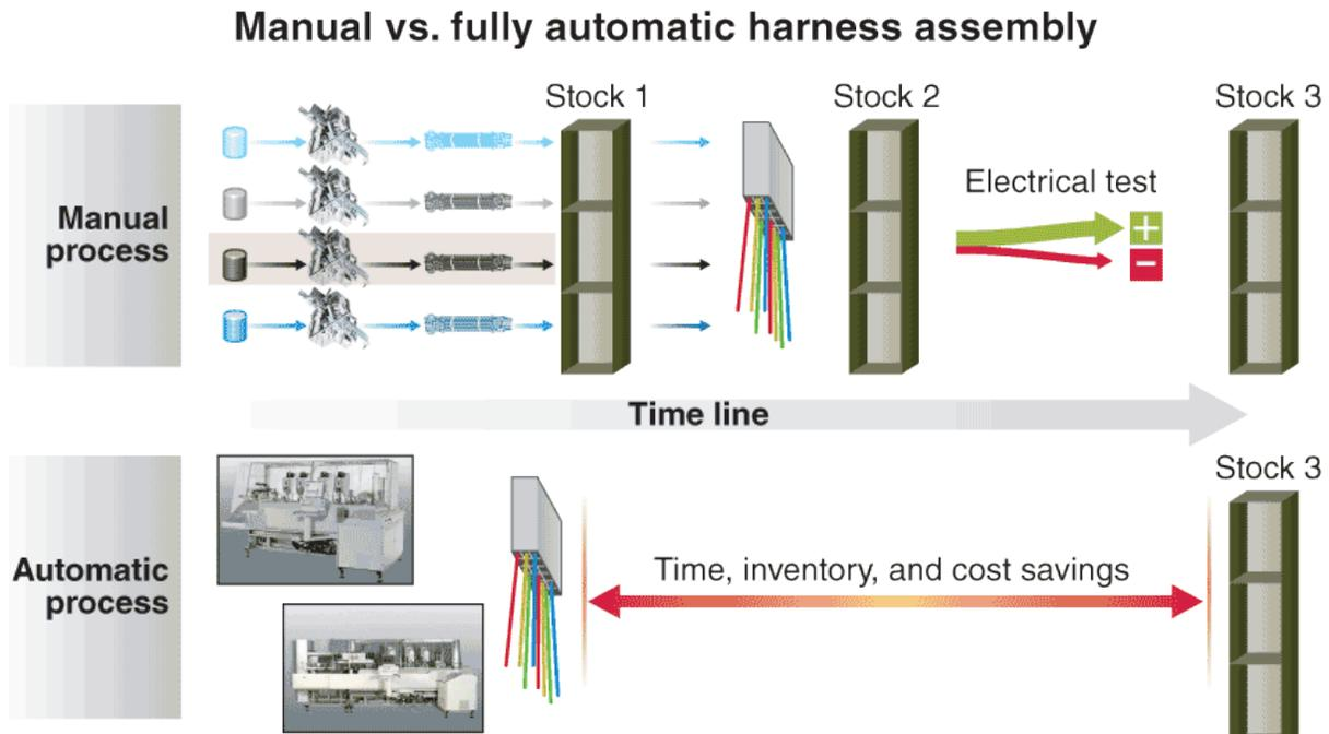
**FIGURE 1.** A comparison of a manual wire harness assembly process using conventional benchtop or semi-automatic machines (top), and a fully-automatic process using harness machines (bottom).
